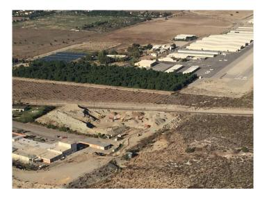
The bad news is that the work is being done with little regard to aircraft operations. Recently we received a call from a flight instructor that said he had to curtail instruction because of poor visibility created by dust (less than visual flight rules). The contractor removing dirt from the stockpile was not employing any dust control (watering). See the photo below.
